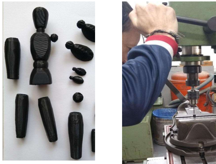
Figure 2 – Printing and drilling of tests based on wooden mannequins
