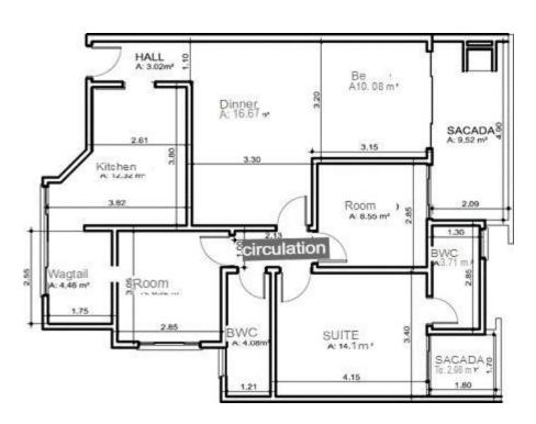
Figure 1: Floor plan of the typical apartment.
