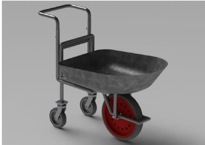
Figure 2 - Proposed concept of an ergonomic wheelbarrow.
