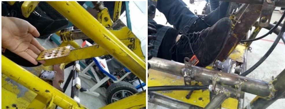
Figure 5: Before and After Adaptation of the Accelerator Pedal
